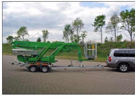
Transport on a purpose built trailer. Up to type 2200, the total weight is less than 3500 kg.
